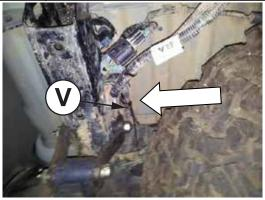
Cable tie the SLT vehicle wiring loom to the vehicle's wiring loom as shown.
