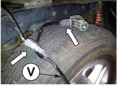
Connect SLT vehicle wiring loom female connector to the fuel filler door actuator and connect the male connector to the vehicle's original connector.
