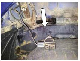
Lower the fuel filler door actuator motor down onto the top of tyre.
