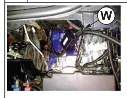
Cable tie the SLT vehicle wiring loom and latching relay to the vehicle's wiring conduit, this is found on the LH inner fire wall below the windscreen wiper water deflector moulding.
