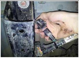
Disconnect the vehicle's wiring harness connector as shown on the inside of the rear LH chassis rail.
