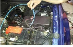
Remove the draw wire from the SLT vehicle wiring loom and tuck the loom next to the fuse box under the other cable conduits.
