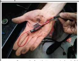
Prepare the front battery terminal end of the SLT vehicle wiring loom as shown opposite, to tape the eyelet terminals down, this is to aid with threading through the SLT vehicle wiring loom to the front of the vehicle.
