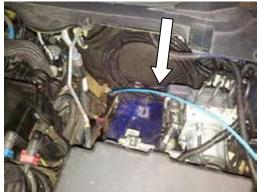
The position of the draw wire should be away from moving parts and underneath any fuel lines, brake lines, air conditioning pipes.
