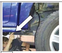
Pull the SLT vehicle wiring loom through and above the fuel tank then along the top of the LH chassis rail.
