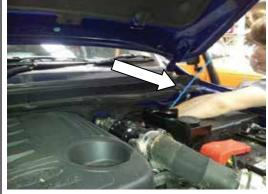
Open the bonnet, feed a plastic coated draw wire down inside next to the LH side fire wall.
