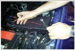
Unravel the previously taped up eyelet battery terminal end of the wiring harness.
