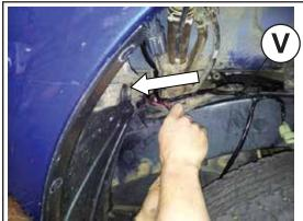
Thread the battery terminal end of the SLT vehicle wiring loom towards the front of the vehicle, along the top of the LH chassis rail via the LH wheel arch.
