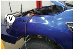
Pull the SLT vehicle wiring loom up into the engine bay.
