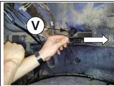
Using the connectors at the rear end for the SLT vehicle wiring loom, thread these in over the top of the vehicle's LH chassis rail and towards the back of the vehicle.
