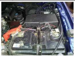
30 Using a 10mm socket drive, connect the red wire to the positive terminal on the battery and the black wire to the negative terminal earthed to the car.
