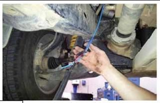
Underneath the vehicle, connect the battery terminal end of the SLT vehicle wiring loom to the draw wire.
