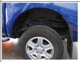
Remove 9 scrivets holding the LH wheel arch liner on the vehicle tub, and remove the wheel arch liner.
