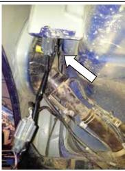
Cable tie the connector back inside the wheel arch and the SLT wiring loom back to the vehicles main wiring loom on top of the chassis rail.
