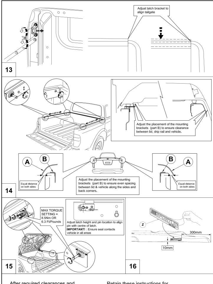
After required clearances and alignement is achieved, tighten all bolts to torque settings stated.
